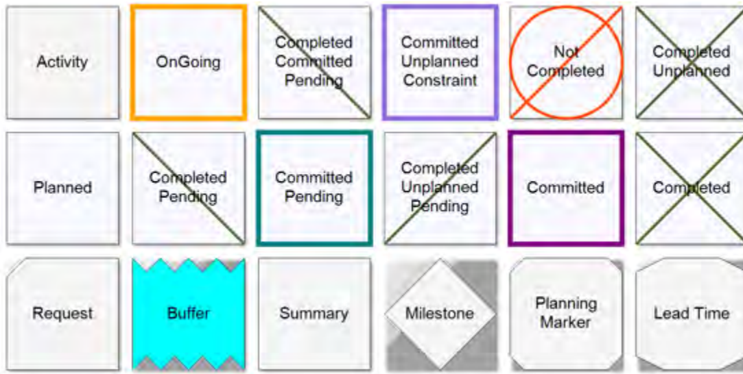
Figure 2. The visual representations of the various task types and their status indicators in vPlanner. (Courtesy: Ghafari Associates)
