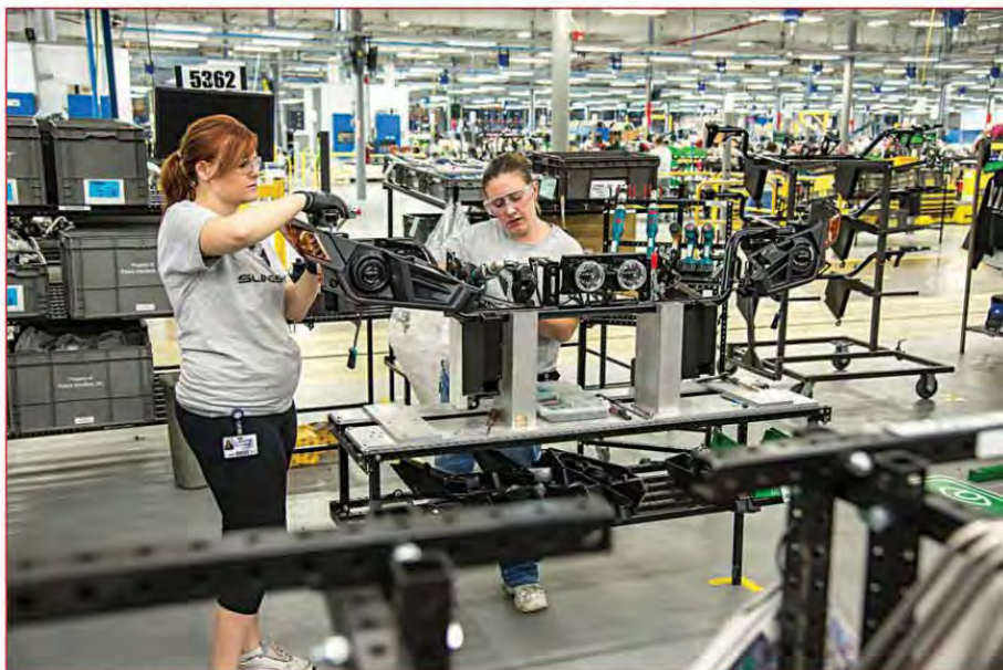
Polaris Spirit Lake addresses error proofing through a variety of built-in poka-yokes and process controls. Photo courtesy Polaris Industries Inc.
