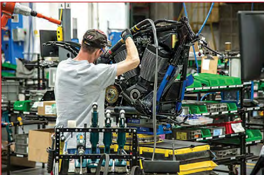
Assembler use DC electric tools for safety-critical and quality-critical fastening applications. Photo courtesy Polaris Industries Inc.
