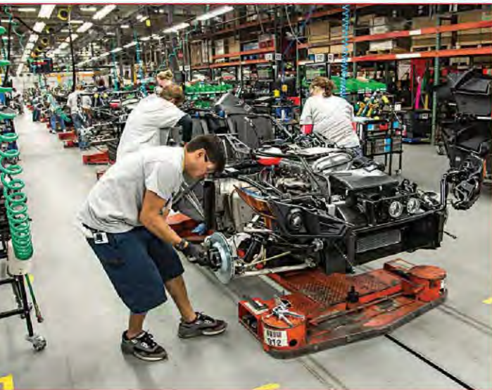
Assemblers at the Polaris Spirit Lake factory build a wide variety of products, including the Slingshot, a cross between a motorcycle and a roadster. Photo courtesy Polaris Industries Inc.
