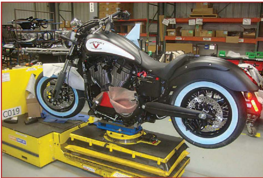
Automated guided carts improve safety, quality and throughput. Photo by Austin Weber
