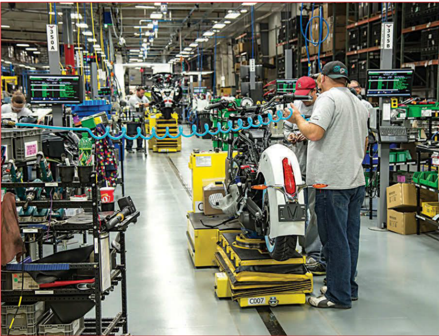
Visual work instructions at every workstation provide a common platform for employee communication. Photo courtesy Polaris Industries Inc.
